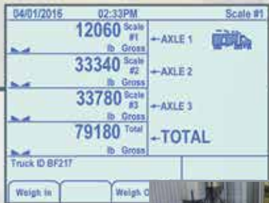
A 32-channel display capability allows viewing of weight on an individual scale and a combination of totalized scales.
